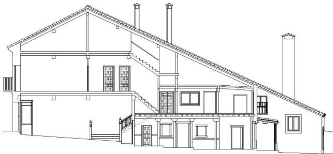
Fig. 6.- Section of the casona del siglo XVII used as an example, where it can be seen the enormous porte de la ceilings of evacuation of smokes.
