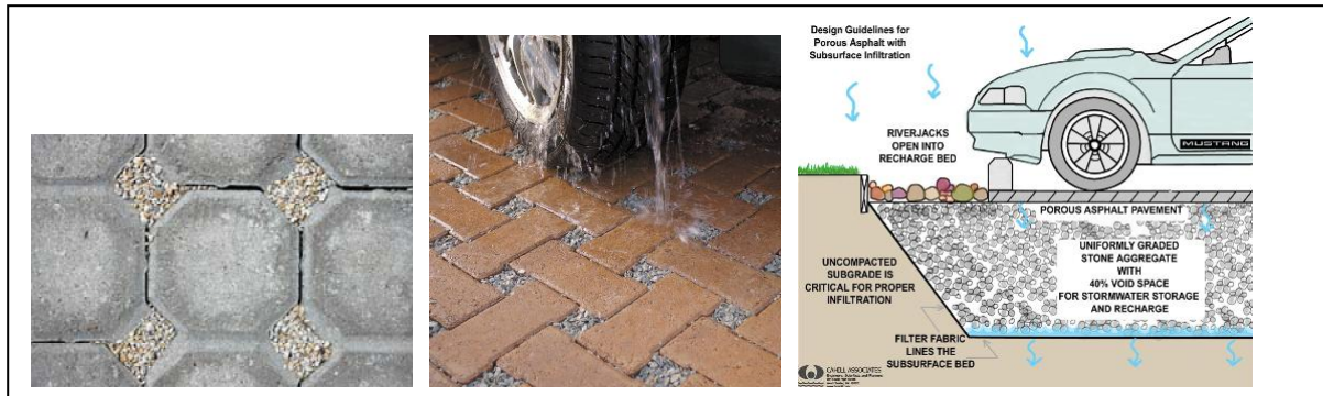
Figure 16: Infiltration Permeable Pavers (Rushton, B.T. 2001: 4)
